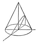
26. When u becomes greater than v, the cutting plane will intersect both nappes of the cone: hence, if a right cone with a circular base be intersected by a plane making with the base of the cone an angle greater than the angle formed by the element and base, both nappes of the cone will be intersected, and the curve of intersection will be an hyperbola.
